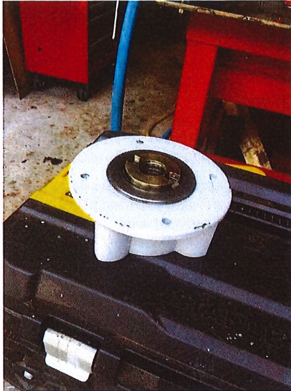
Figure 4: Top view of bush (inner) and mounting (outer).
