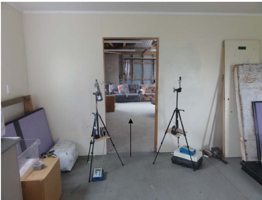
The photograph above shows air sampling instruments set up either side of a doorway from a kitchen into lounge area in the garage. To simulate fume emissions from the firing of FX ammunition an officer stood in the doorway and fired into the lounge. An arrow shows the direction of firing the handgun.
