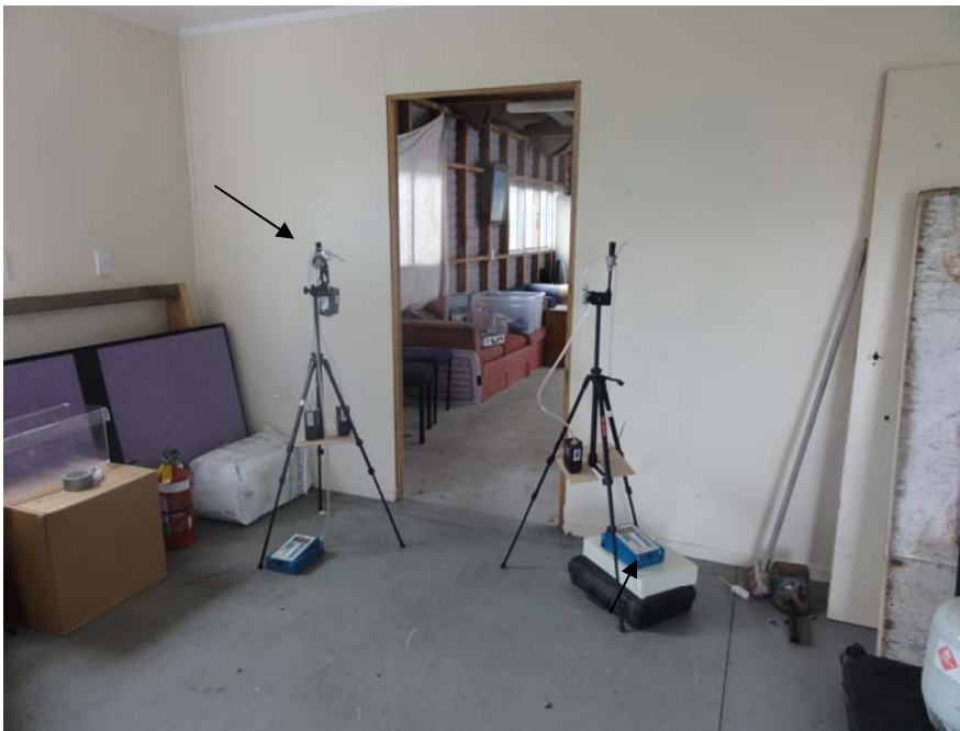
The photograph above shows air sampling instruments set up inside a garage that is adjacent to the building containing the upper indoor firing range at the Royal New Zealand Police College. See the arrows.
