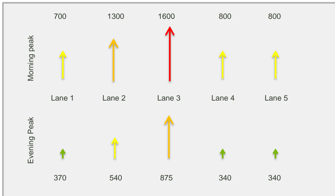
Figure 2-9 SH16 Eastbound Approach and Demand Lane Balance
