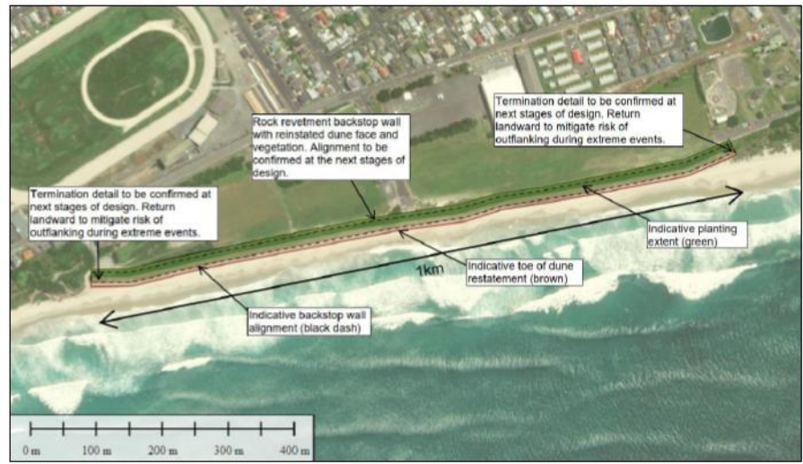
Figure 4-7: Concept sketch of backstop rock revetment.
