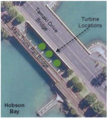
The causeway site is a less than 325 m from the Parnell Baths complex. The design would include a free-standing, enclosed, generator control panel near the tidal causeway, with an underground cable along the Tamaki Drive road reserve, then rising above ground and passing under the wooden pedestrian rail over-bridge en-route to the plant room on the south-west corner of the baths
