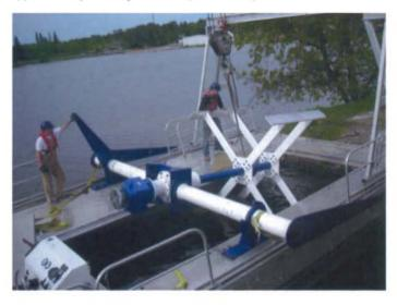
New Energy Ltd advises that the 'low flow' 25kW vertical axis turbines mounted on an overhung cradle support should prove to be best for the Tamaki Drive causeway channel.
