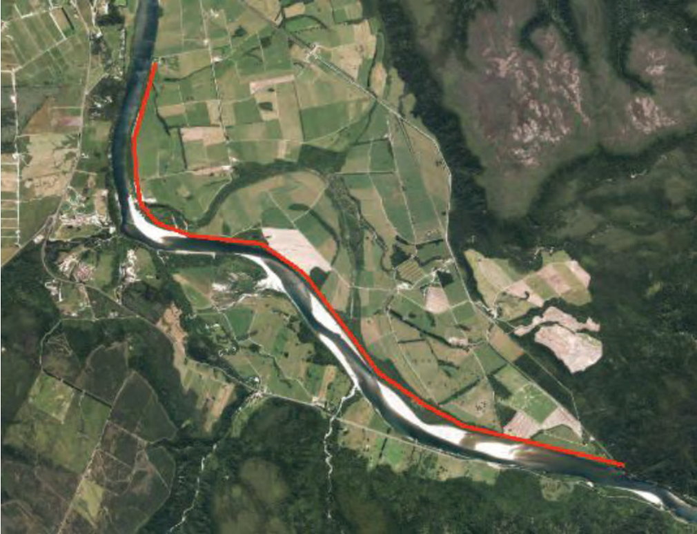
Figure 5-5: Location of 'glass wall' inserted into model to prevent overflow down the Orowaiti
