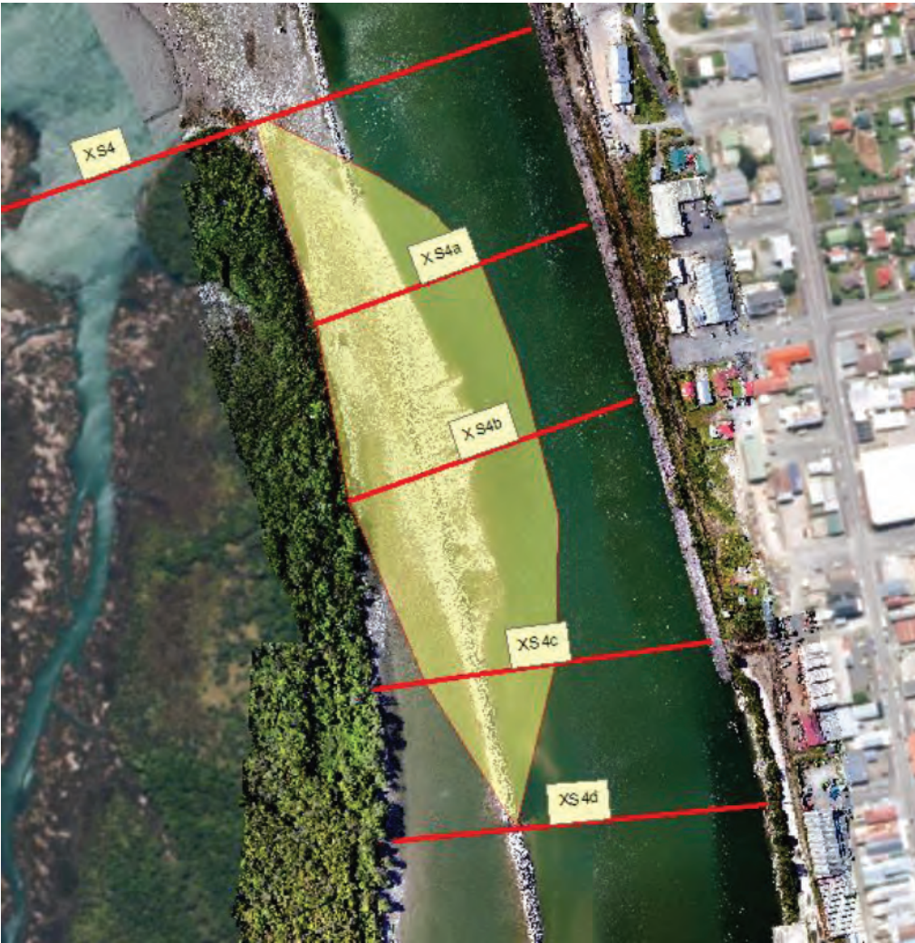
Figure 5-3: Modelled hypothetical gravel build-up between XS4 and XS5 (yellow area indicates exposed gravel)
