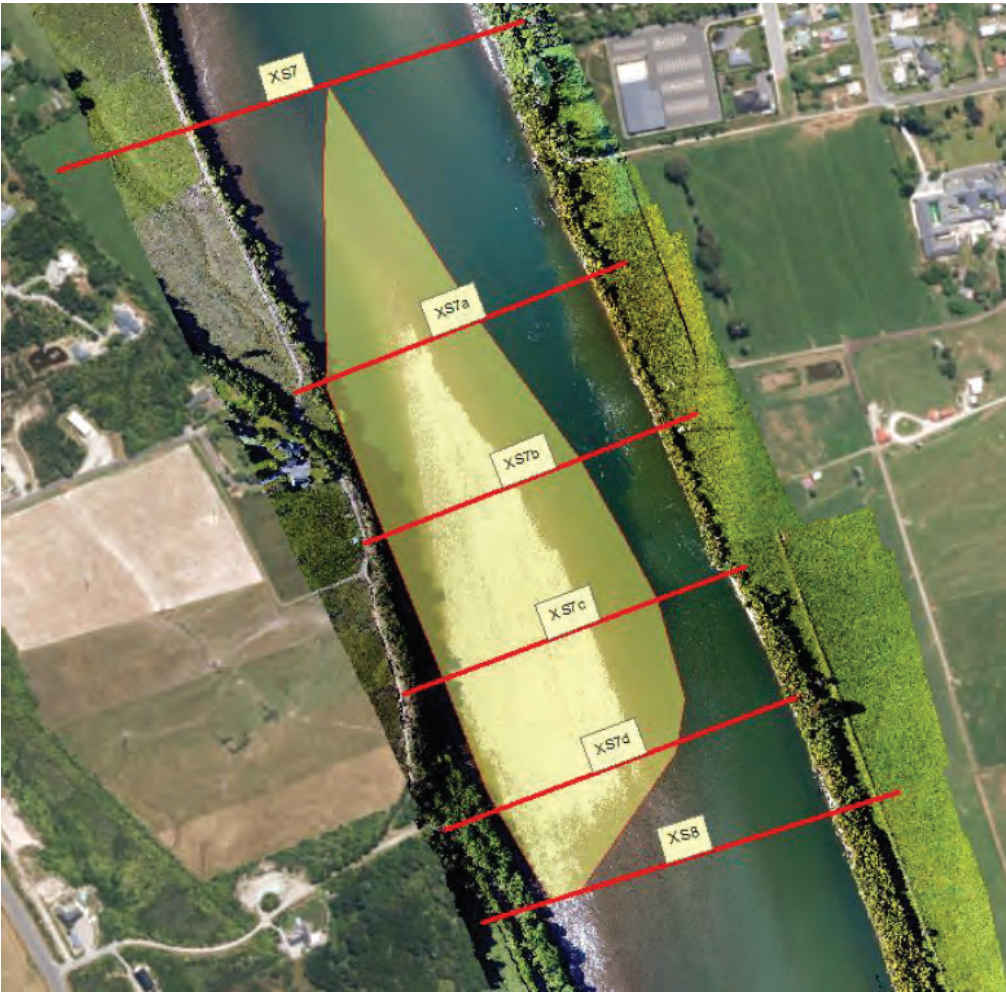
Figure 5-4: Modelled hypothetical gravel build-up between XS7 and XS8 (yellow area indicates exposed gravel)
