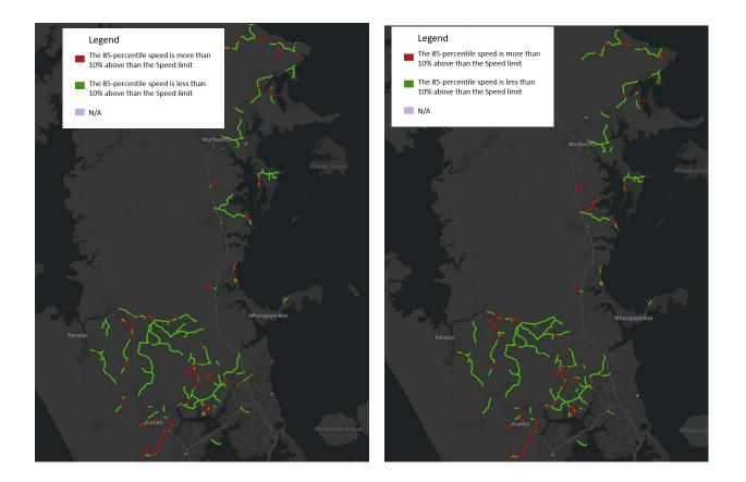
Figure - Compliance map North Auckland Direction 1 on Left and Direction 2 on right (February 2022)
