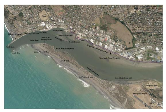
**Figure 4:** Photo of the area showing the location of key river management infrastructure in the lower Whanganui River. Note Stage 3 of the project relates to structures upstream of the Tanae Groyne on the same side of the river, including the South spit embayment, south spit Groynes and concrete walls. Map created in 2017.
