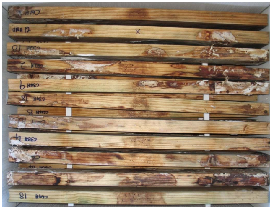
Figure 1 – Decay on copper naphthenate treated samples after 159 weeks exposure, HMC tank 1, layer 5, (2 nd from top). Extensive decay mycelium on the samples including on treated surfaces, still active and progressive.
