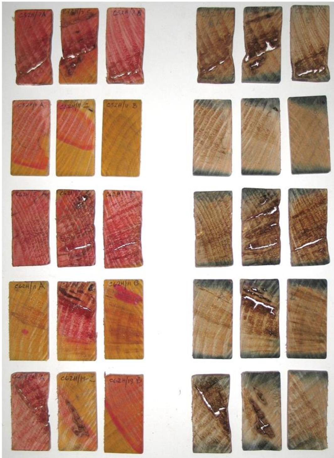
Figure 13 – Decay and preservative penetration in copper naphthenate treated samples (HMC tank treated on two edges). All samples contain extensive decay although in the second from top sample it was mainly at one end. There was limited preservative penetration and decay was active up to and through the treated area.
