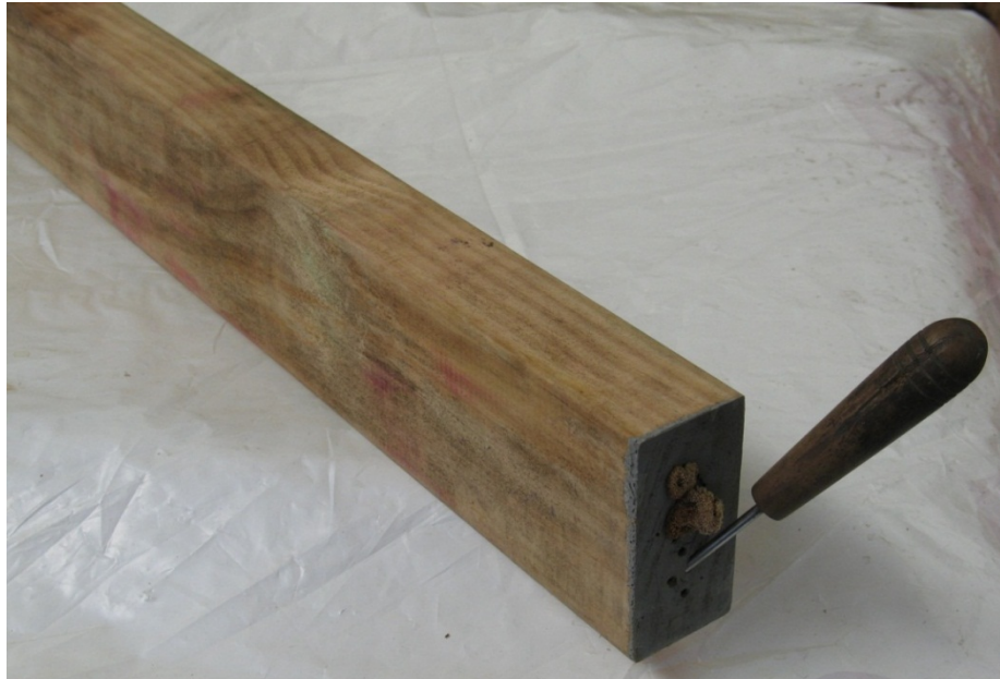
Figure 19 – LMC sample C64L/5 treated with copper naphthenate on four sides after 157 weeks exposure. This was in layer 5 near one side of the stack and would have not been wet by condensation drips hence its moisture content would have been between 25% and 30% for the duration of the trial. There were decay fruiting bodies at one end and decay extending full length of the sample through the centre. There was no decay on the exterior of the sample except what appeared to be an inactive area at the point where the original decay feeder block had been attached before treatment.
