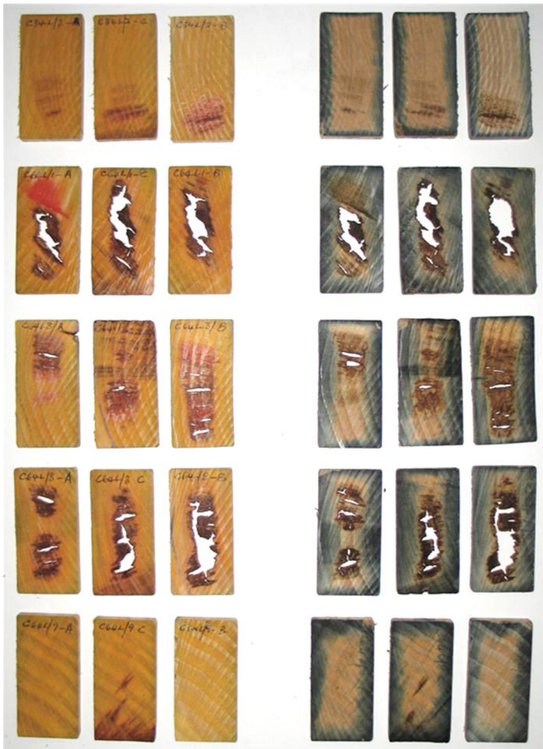
Figure 15 – Decay and preservative penetration in copper naphthenate treated samples (LMC samples treated on four sides in Table 4). There is limited copper penetration and there was active decay through the centre of the top four samples. Decay in the bottom sample was limited to the central section on one edge and had spread slightly from the area where the original decay feeder block had been attached.
