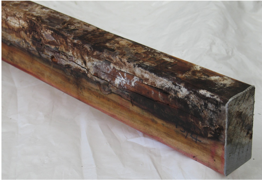
Figure 23 – HMC sample B61H/12 treated with boron on one edge after 159 weeks exposure. There was severe decay throughout the sample, away from the treated edge. This was typical of many of the samples in the group that were treated with boron on one edge only.
