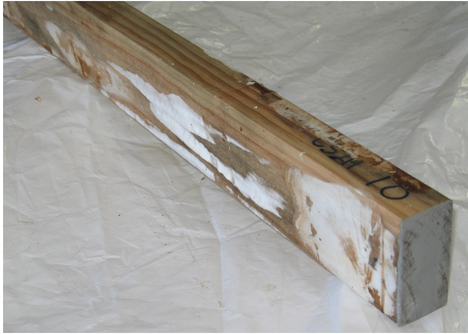
Figure 21 – HMC sample C32H/10 treated with copper naphthenate on two edges after 159 weeks exposure. Decay has spread along the length of the sample including over the treated edges. It was severe in patches and the sample rating was 6 (30-50% of the cross section decayed). MOE had declined by 11% during the exposure period.
