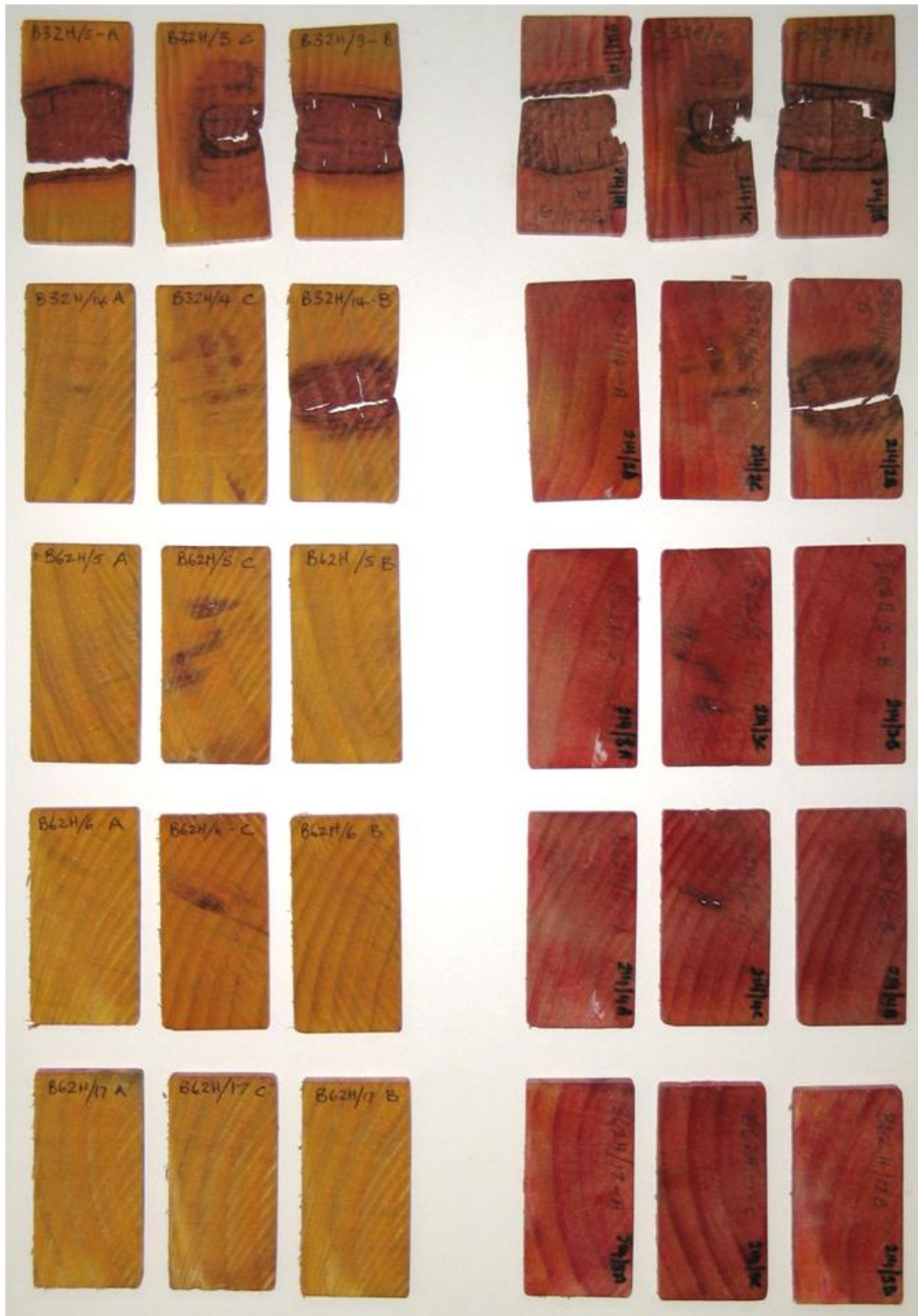
Figure 14 – Decay and preservative penetration in boron treated samples (HMC tank treated on two edges). All samples contain some decay although in the three lower samples it appeared to be from the original feeder block and was inactive. The reagent test colour suggests that the boron had spread through the sample from the two edges that it had originally been applied to.
