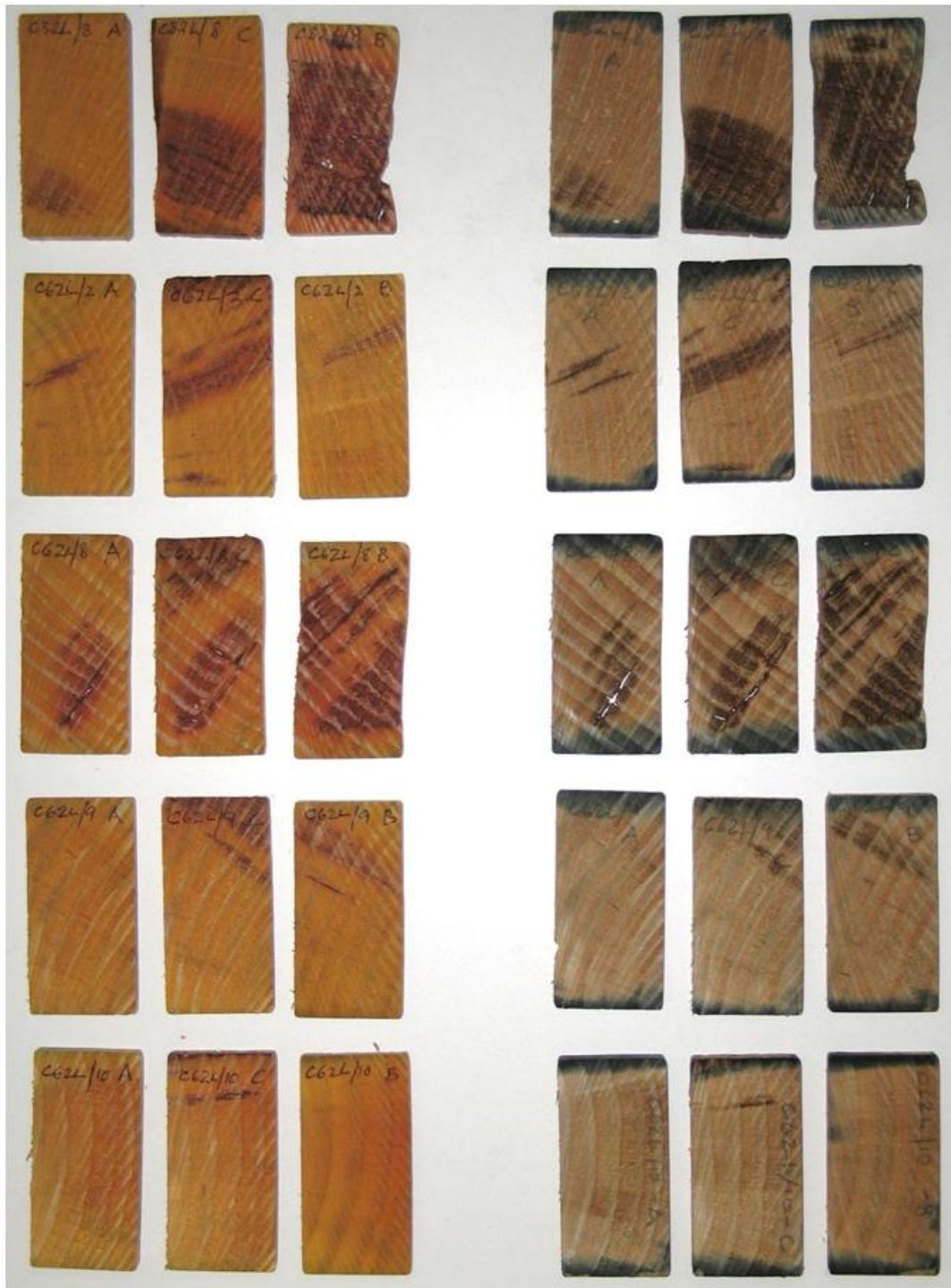
Figure 17 – Decay and preservative penetration in copper naphthenate treated samples (LMC stack treated on two edges). All samples contain some decay although the decay in the bottom two samples was from the original feeder block and appeared inactive. There was limited preservative penetration and decay was active up to the treated area.
