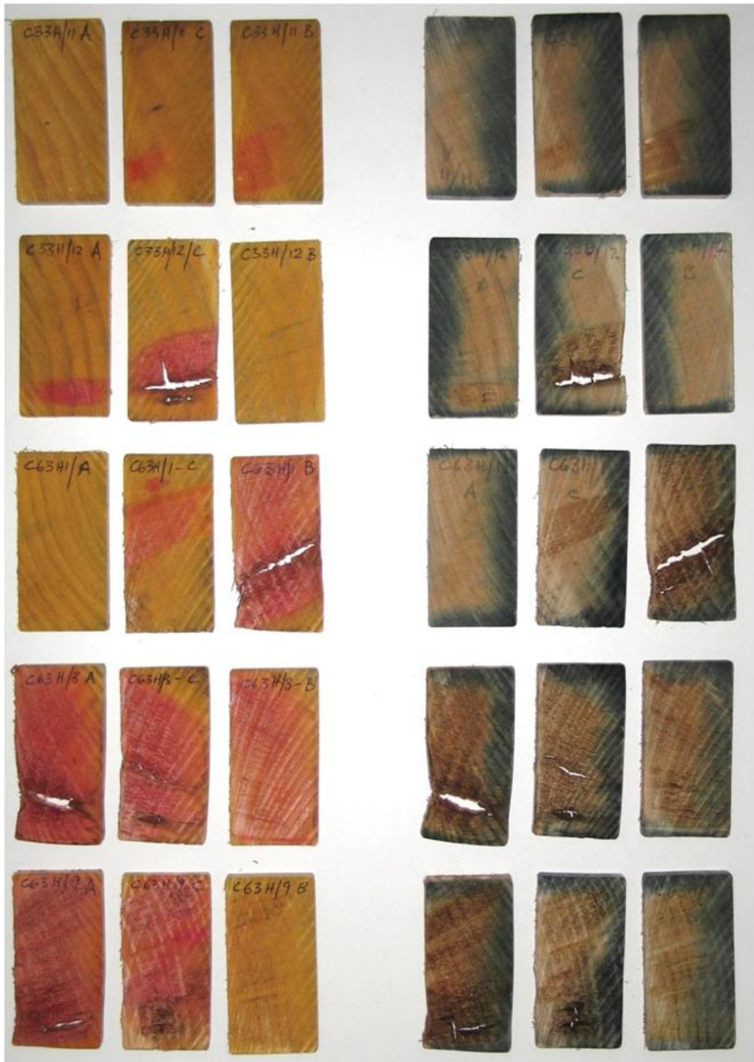
Figure 11 – Decay and preservative penetration in copper naphthenate treated samples (HMC tanks treated on one face and two edges). Preservative penetration is limited and all samples contain some decay extending into the treated areas.
