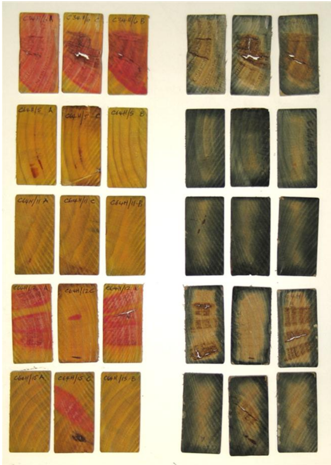
Figure 9 – Decay and preservative penetration in copper naphthenate treated samples (HMC samples treated on four sides in Table 6). The samples on the left have been sprayed with methyl orange reagent which turns a pink-red colour where there is active decay. The samples on the right are matched with the decay test samples and have been sprayed with rubeanic acid reagent which turns blue-black in the presence of copper. The three biscuits in each set are from the same sample, the central “C” sample from the original decay feeder block position, the “A” and “B” samples 150 mm from each end. There is limited, variable copper penetration and active decay in three of the samples.
