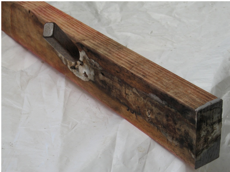
Figure 24 – HMC sample B32H/13 treated with boron on two edges after 159 weeks exposure. There was a strip of severe decay through the centre of the sample but this had not spread to the treated edges. This sample was in the top layer of the tank and it is likely that boron loss would have been greater than for samples lower in the tank. MOE for this sample had reduced by 23% over the exposure period due to this decay (rated 6, 30-50% of the cross section).
