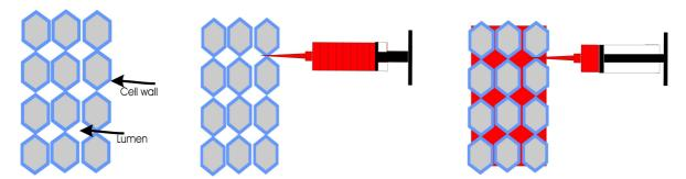
The idea being to inject the wood matrix with polymer precursor viz. monomeric and then curing the material free-radically to form a polymer network.
