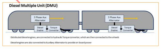
Figure 5-1: Characteristics of a DMU with diesel-hydraulic transmission
