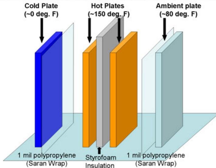
All metal plates coated with high emissivity ( $\epsilon=0.99$ ) Krylon flat white #1502
