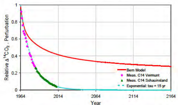
Figure 5. Decay of perturbation predicted by the Bern Model (Red Graph) as calculated from (15). Also shown is the observed ^{14}C decay (Circles and Triangles) and an exponential fit with a decay time \tau = 15 \text{ yr} (Dashed Blue).
