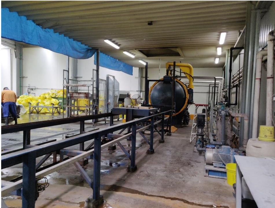
View of the interior of the processing facility, the autoclave is the black machine in the centre.
