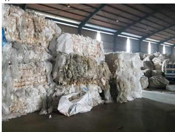
Baled plastic film at receiving point of facility
